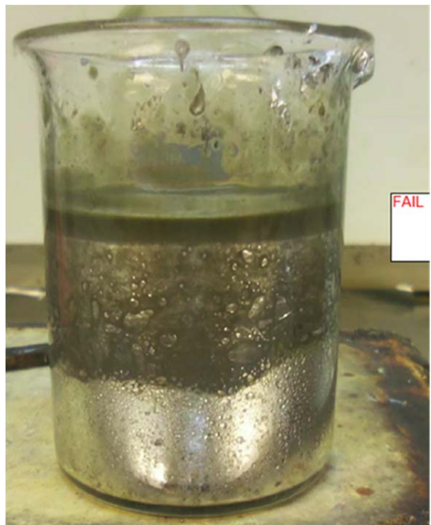
Figure 7. Qualitative Dross Inclusion Recycled SAC 0307
