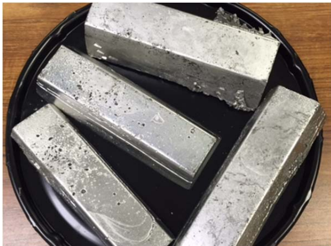
Figure 1. Cast Ingots of Recycled 63/37 Alloy
